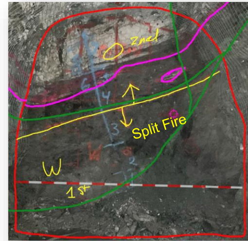
Split fire opportunity identified using ore/waste calculations (Lithology above sampling domains below).
