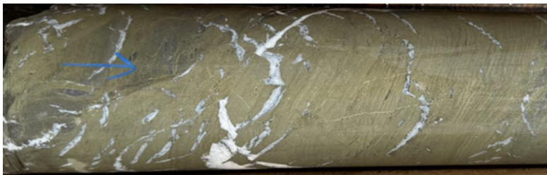
Figure 4: CD24-002 at 119.8m; laminated massive sulphides, predominant brassy chalcopyrite thinly interbedded with pyrite with white carbonate veins (assayed 13%Cu + 21.1 g/t Ag).
