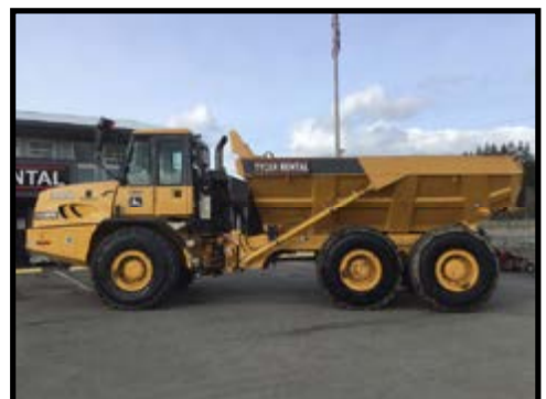
2013 Deere 300D II ..... #88-30043 7531 Hrs, 30 Ton Articulated Truck, 6X6, IT4 Diesel Engine, 23.5R25 Tires Chehalis, WA ..... $169,500
