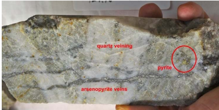
Figure 4: Aurora Prospect, West Pogo Block, Hole #1 (20AU01) 127.16m - 127.3m quartz veins, arsenopyrite and pyrite in paragneiss. Grade 0.19g/t Au, >10,000ppm As, 9.4ppm Bi, 1.13ppm Te.
