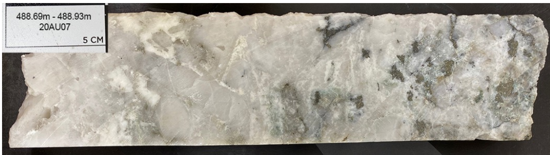
Figure 3: Aurora Prospect, West Pogo Block, Hole #7 (20AU07) 488.69m – 488.93m quartz vein with fuchsite, arsenopyrite, pyrite and pyrrhotite included in a 7m thick interval of quartz vein.
